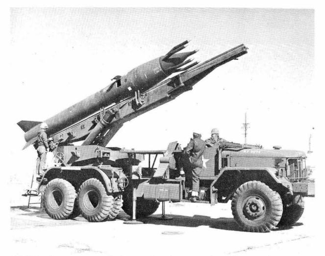
FIVE-FUZE configuration on a modified Honest John rocket was tested recently at Tonopah Test Range as part of a project for the Army's Harry Diamond Laboratory. Diamond is the developer of a fuze for the Army's General Support Rocket. The hydra-headed nosetip provided testing for five separate fuzes on a single rocket. Test director was Wayne Lathrop (1173); Harold Rarrick was test project manager.
